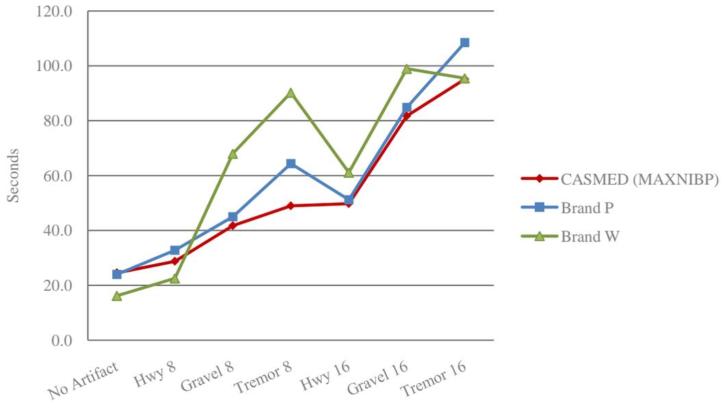
Fig. 5 – Average Time to Measurement at Each Artifact Level for All NIBP Units Tested
