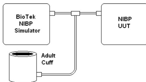
Fig. 1 – Motion Artifact Comparison Testing Equipment Setup
